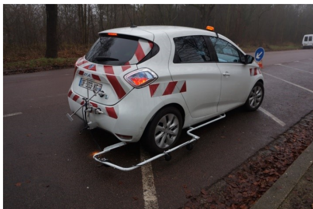
Figure 10. CPX measuring equipment; City of Paris.
